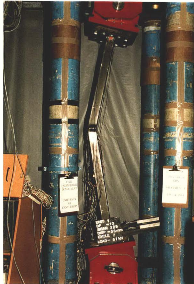
Figure 3.12: Specimen #1 subjected to a contraction of -39.6 mm, axial ductility of -8.56 in the seventh cycle. Overall and local buckling are evident.
