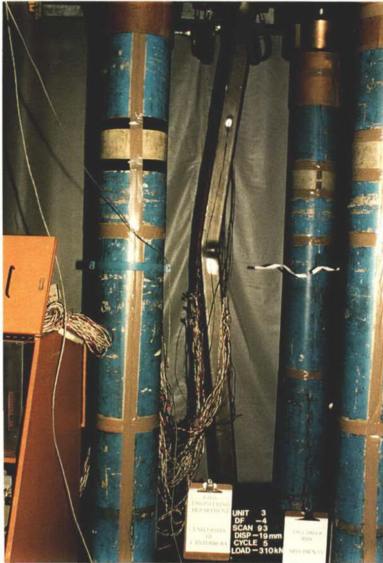
Figure 3.21 Specimen #3 in cycle 5 showing overall and local buckling
