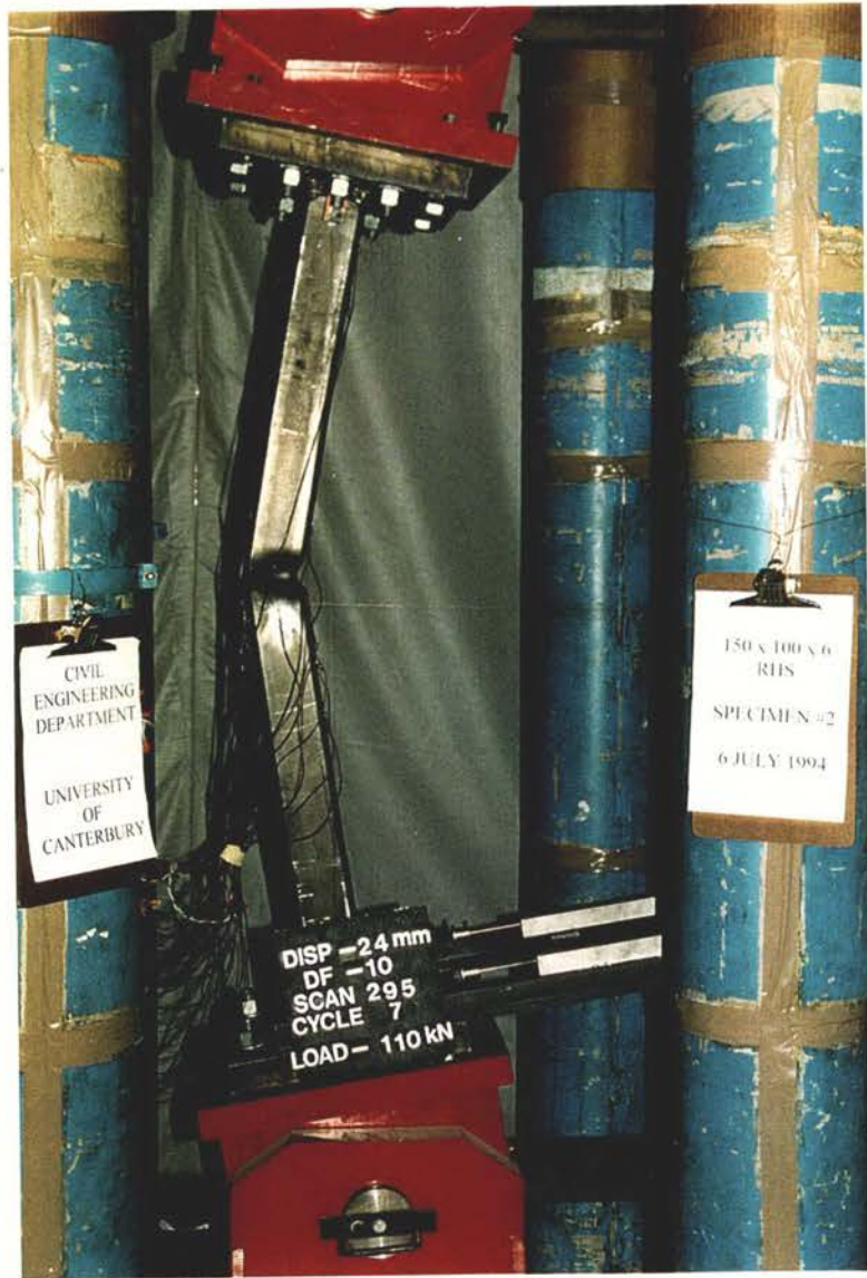
Figure 3.17 Specimen #2 in cycle 7 showing overall and local buckling
