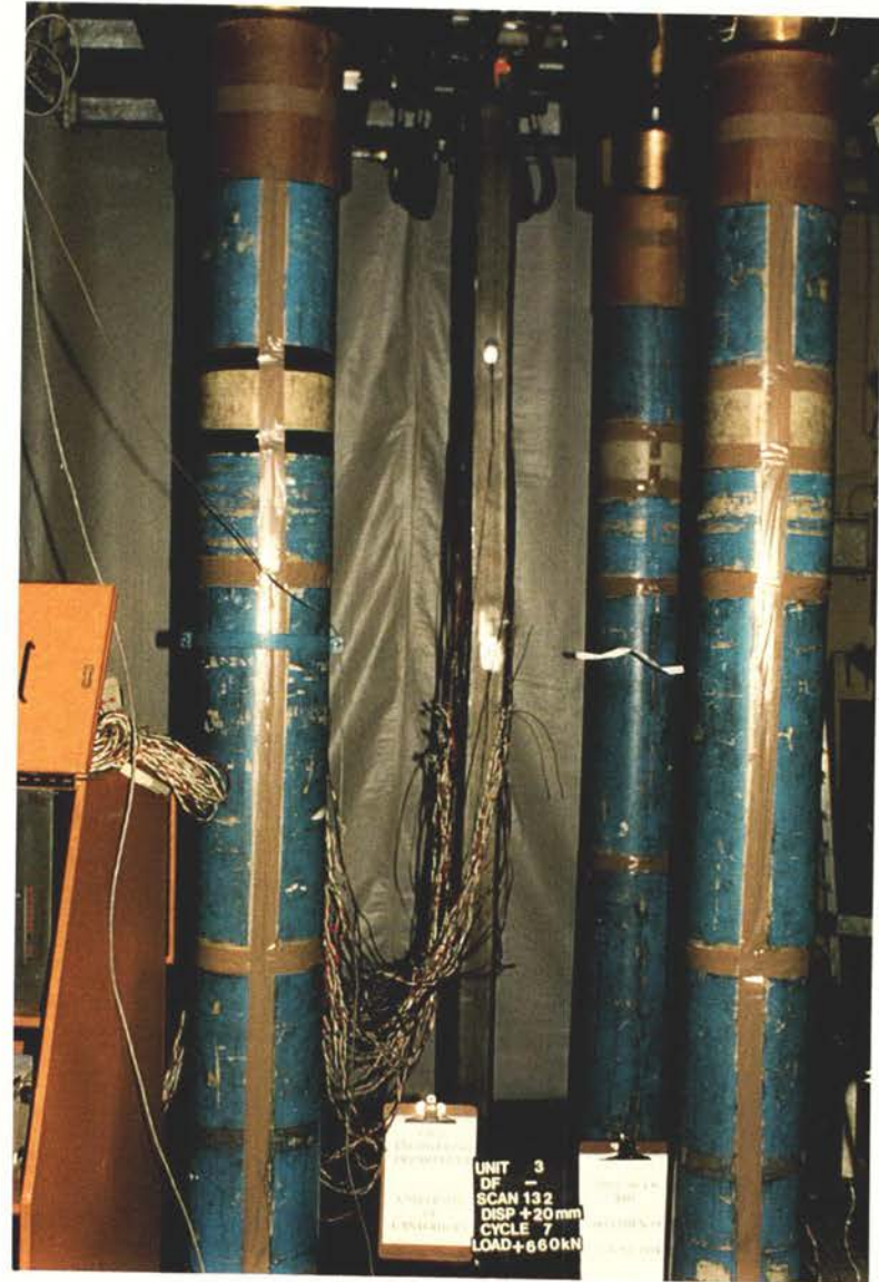
Figure 3.24 Specimen #3 in cycle 7 near the end of the test, showing a crack at the mid-height of the member
