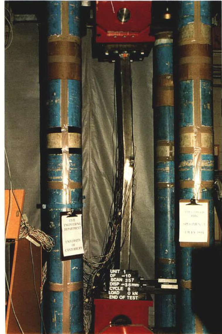
Figure 3.14: Specimen #1 at the end of the test showing the fracture on one side of the member at mid-height.
