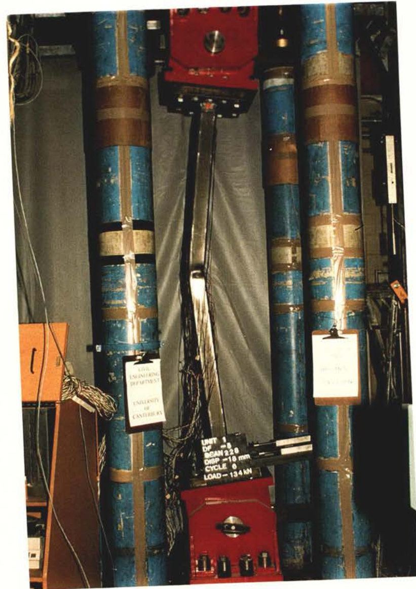
Figure 3.10 Specimen #1 subjected to a contraction of 19.4mm, showing overall buckling and local buckling
