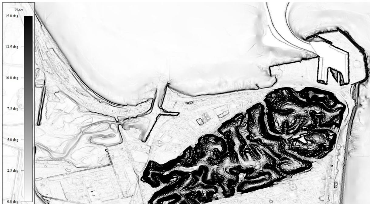
Figure 3.1 Details of the nearshore bathymetry of the digital elevation model (DEM), including Napier Port and the Ahuriri Estuary revealed with slope shading imaging. The figure shows the local slope in degrees. This method of visualising the DEM highlights the parts of the region with steep slope that are most likely to stop or inhibit the tsunami inundation (e.g. Bluff Hill).
