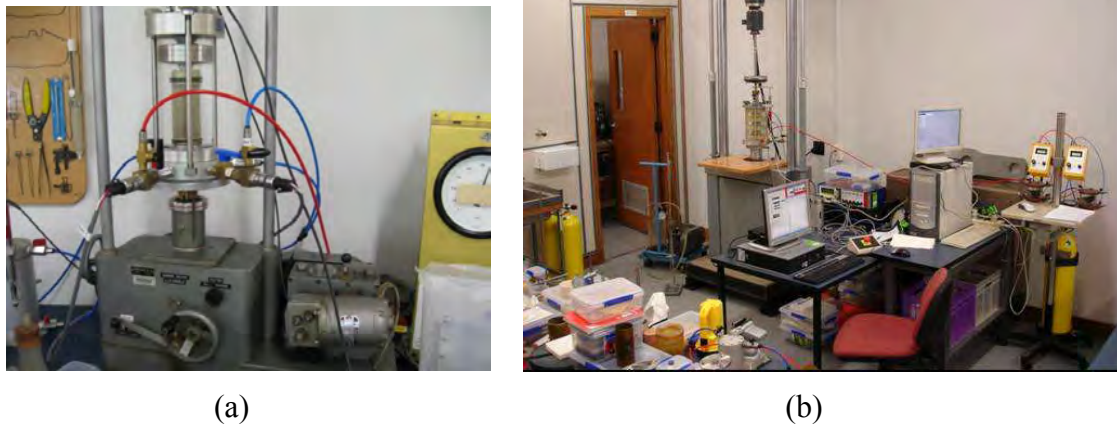
Figure 3.4: Triaxial machines used in the tests: (a) for monotonic CU tests; and (b) cyclic undrained tests.
