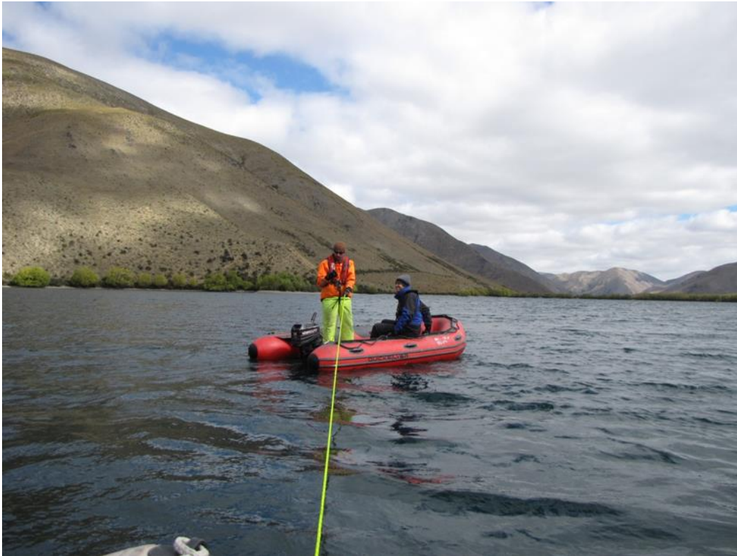
Figure 5.1 Inflatable boats used to survey and core within Lake McRae. The lake has a maximum depth of c. 43 m. The trace of the Clarence Fault is seen by the green vegetation line behind the boat.
