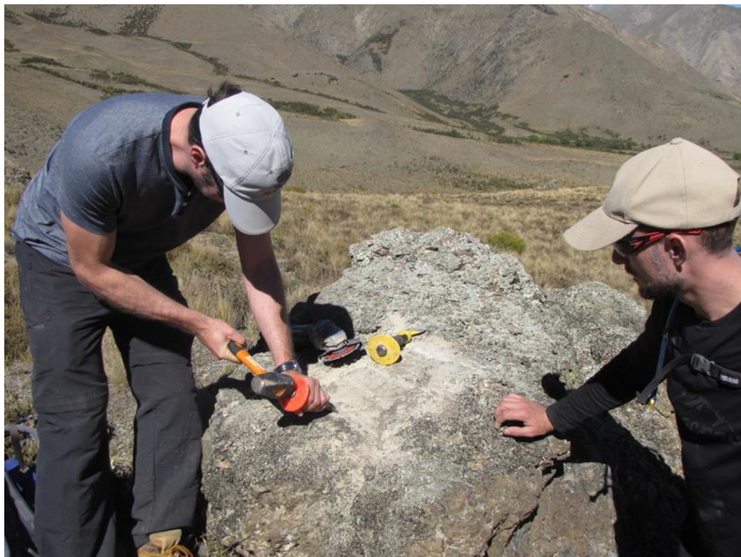
Figure 4.6 Rock sampling technique on the LS1 landslide deposit. A square area of north-facing surface rock was prised out with a portable rock saw and manually with a hammer and chisel (sample LS1-B3).
