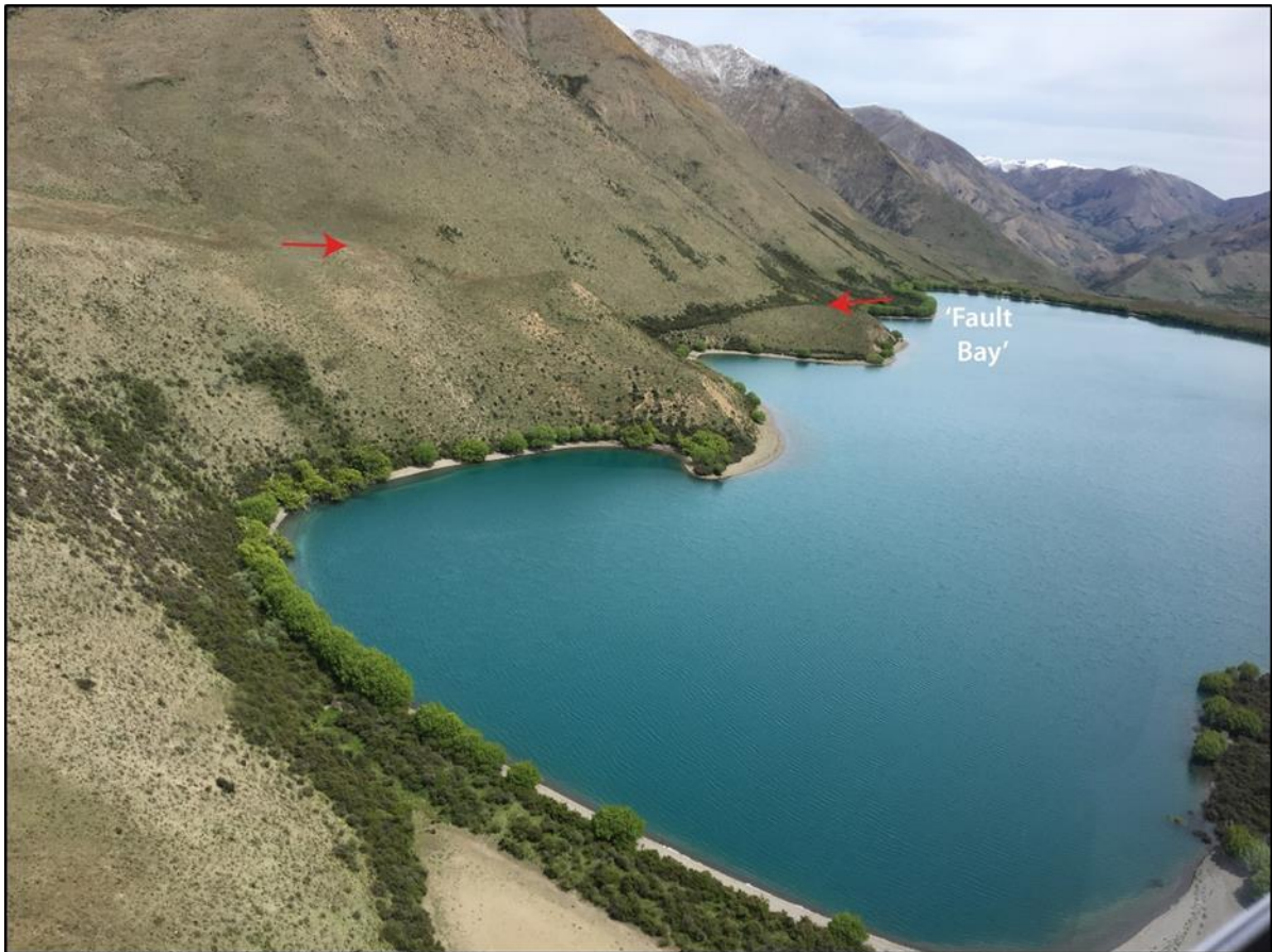
Figure 2.4 Oblique aerial view of the southern side of Lake McRae. The vegetation lineament running along the base of the range highlights the trace of the active Clarence Fault (red arrows). Photo: Matt Hill.
