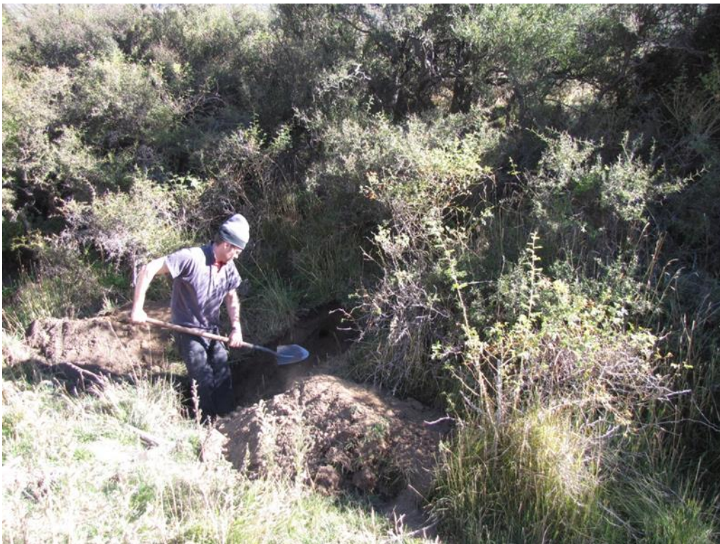
Figure 3.3 Location of the trench dug across the trace of the Clarence Fault into the toe of a shutter scarp. Location of the trench dug across the trace of the Clarence Fault into the toe of a shutter scarp. The uphill-facing scarp at this location is c. 4 m high here.
