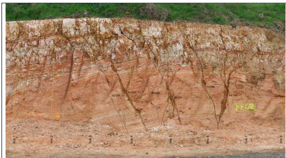
Figure 17. Exposed face within an excavation at Rototuna showing faults within the Kukutaruhe Fault Zone.
