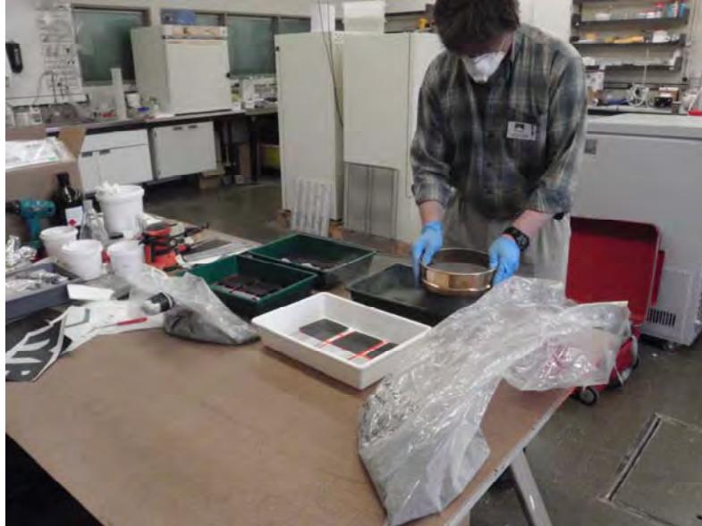
Fig. 5: Allan Scott using a sieve to distribute dosed pseudo-ash over samples of roofing material for one-month trial in environmental test chamber (Photo: C. Stewart)
