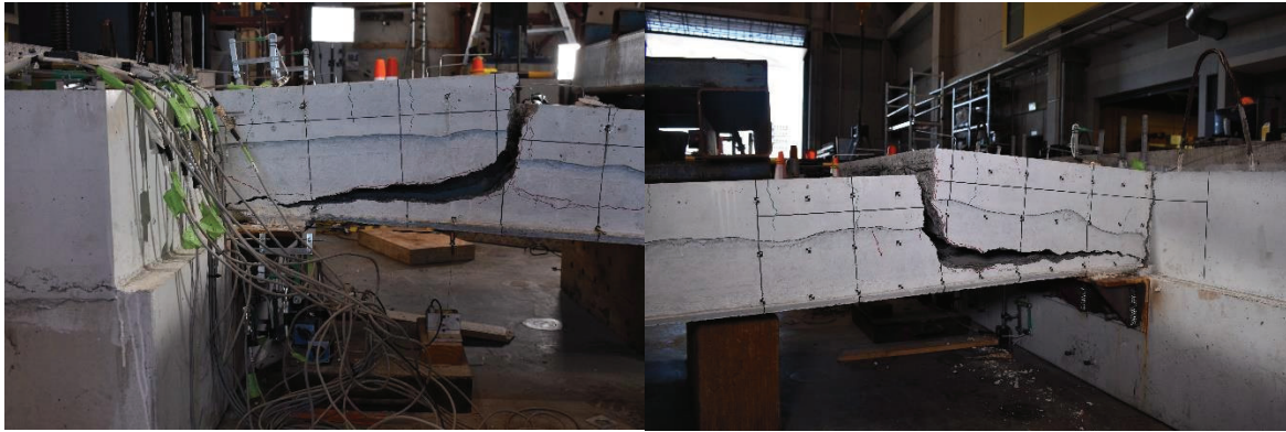
Figure 26: Unit Connection at -6.0% drift – End of Test
