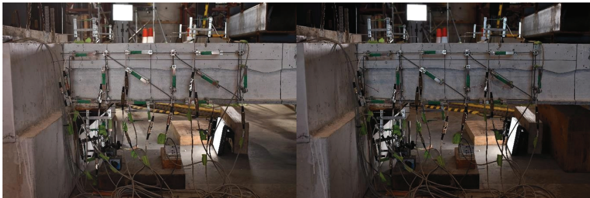
Figure 19: East Side of Specimen 4 Directly Prior (Left, -1.0% Drift) and After (Right, -1.6% Drift) NM Crack Initiation
