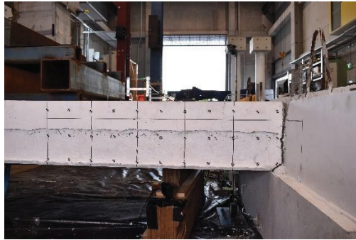
Figure 9: Specimen 1 Residual Crack after Full Cyclic Protocol Up to \pm 4.5\% Drift
