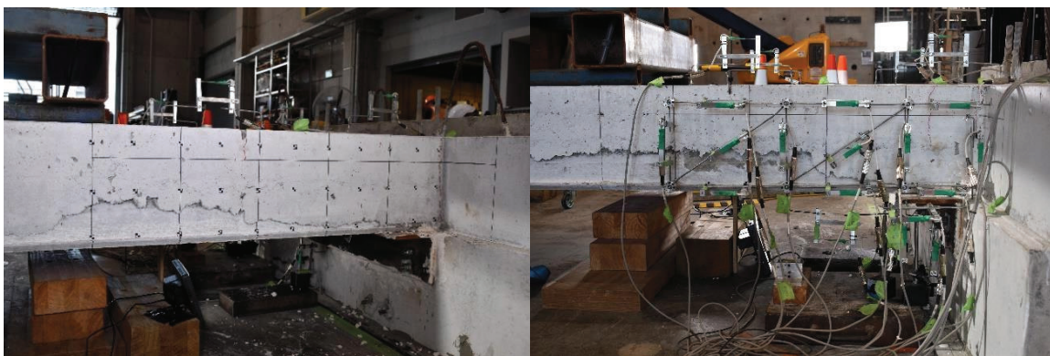
Figure 112: Specimen 3 at -0.53% Drift – Initial Crack Propagation (West – Left, East – Right)
