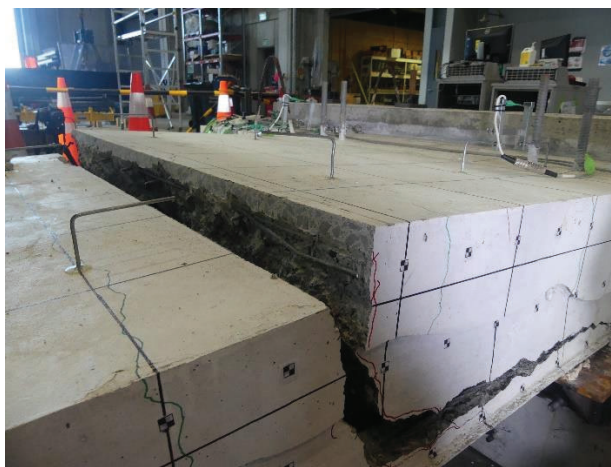
Figure 27: Snapped Mesh visible at Test End
