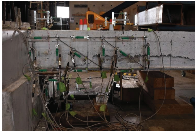
Figure 14: Specimen 3 at -1.25% Drift – Critical Crack Propagation (East Side)
