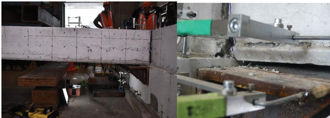
Figure 36 Specimen 6 at +3.0% Drift (West – Left) and LOS on Eastern Side at +3.0% Drift
