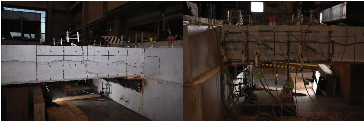
Figure 20: East Side (Left) and West Side of Specimen 4 (Right) at Second -2.0% Drift Peak Displacement Cycle
