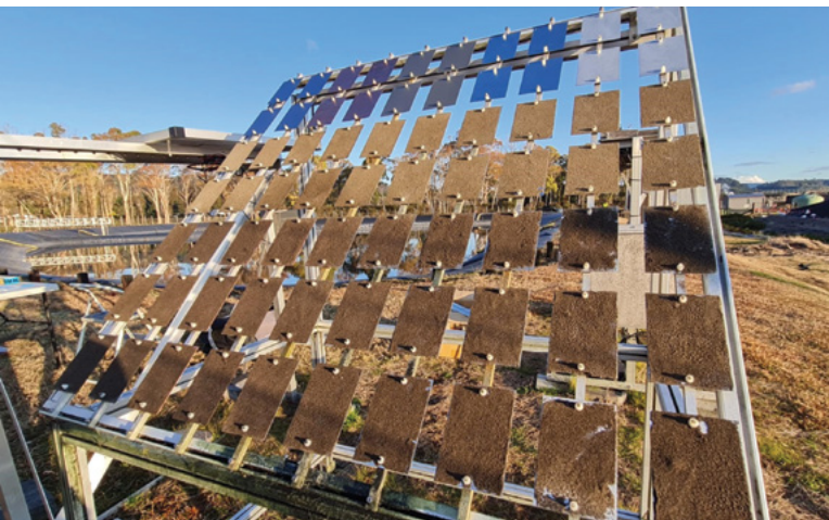
Volcanic ash-coated samples at Rotorua wastewater treatment plant near Sulphur Bay
