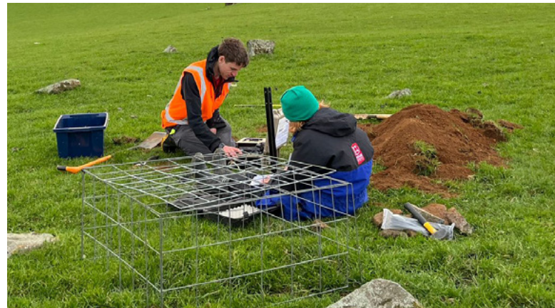
Researchers installing seismometers in Southland
